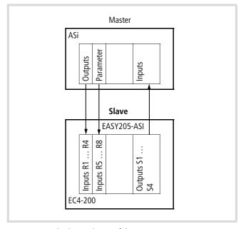
Figure 103: Cyclic data exchange of the EASY205-ASI
