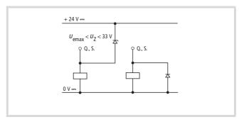
Figure 26: Inductive load with suppressor circuit
