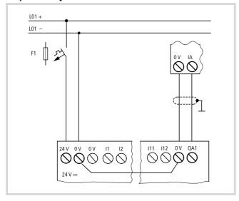
Figure 28: Setpoint entry for a drive
