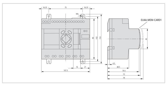
Figure 115: Dimensions in mm (specified in inches → table 24)
