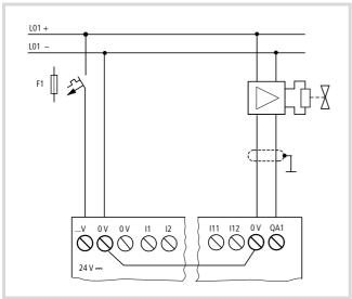
Figure 27: Connecting servo valves
