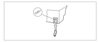
Figure 12: Inserting a fixing bracket
