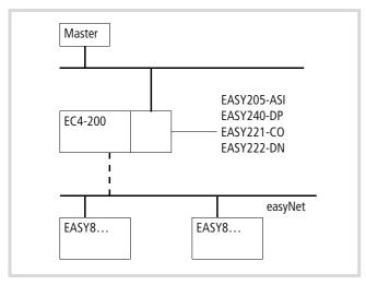
Figure 102: EC4-200 wih network connection
