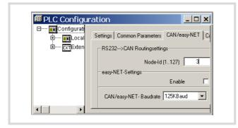
Figure 85: CAN Master routing settings
