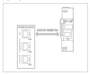
Figure 6: Connecting the PLC with XT-RJ45-ETH-RS232
