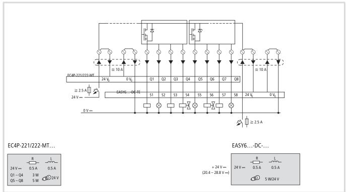
Figure 25: Transistor outpus EC4P-221/222-MT..., EASY6-DC-TE
