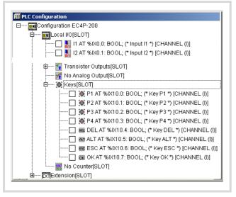
Figure 5: Inputs of the rocker and function buttons
