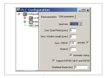
Figure 86: CAN Master, ID for basis communication
