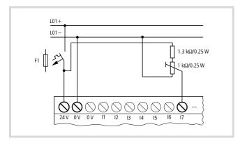
Figure 18: Setpoint potentiometer with upstream resistor
