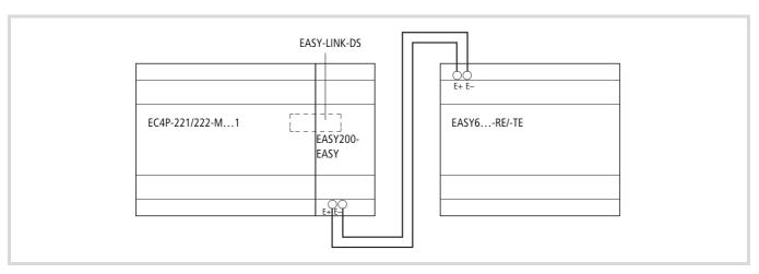
Figure 34: Connecting remote expansion units to the EC4-200
