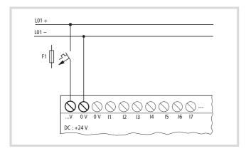
Figure 15: Connecting the power supply
