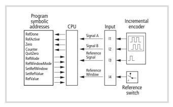
Figure 46: Input/output signals of the incremental value counter
