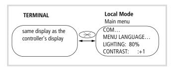
Figure 101: Toggling Terminal mode ↔ Local mode
