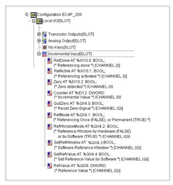
Figure 45: Input/output signals of the incremental value counter
