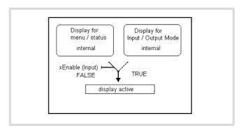
Figure 92: Changing from Status display ↔ Entry/output mode
