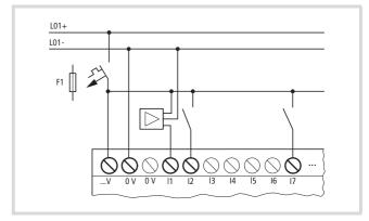
Figure 16: Connecting digital inputs
