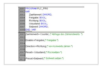
Figure 41: Programming inputs/outputs of the 32-bit counter
