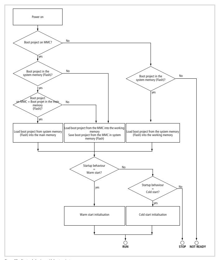
Figure 39: Startup behaviour with boot project
