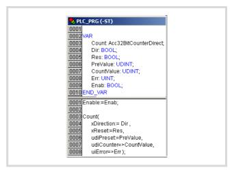
Figure 43: Program with FB for 32-bit counter
