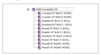
Figure 44: Inputs/outputs of the 16-bit counter 0 and 1
