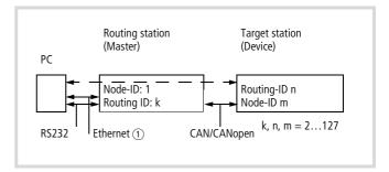
Figure 84: Routing via ID1 (XC..., EC4-200 or MFD4)
