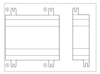
Figure 13: Screw fixing the devices
