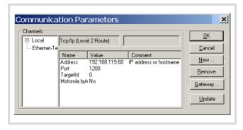
Figure 79: Communication parameters with IP address
