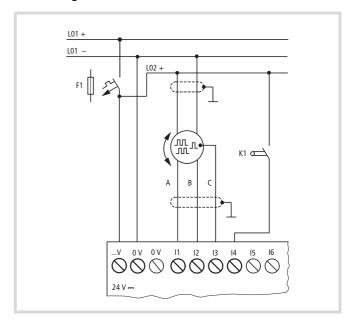
Figure 23: Connecting the incremental value encoder
