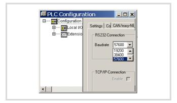
Figure 74: Specifying the CPU's communication settings
