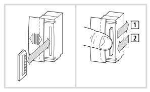
Figure 31: Fitting/removing the memory card
