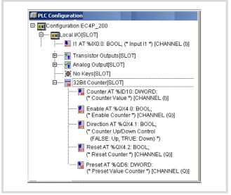
Figure 37: Configuring a counter (32-bit)
