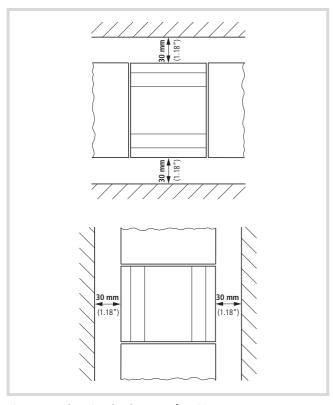
Figure 10: Observing the clearances for wiring
