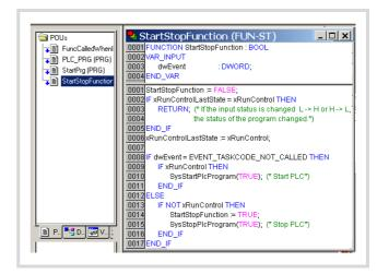
Figure 113: Function that monitors the input
