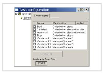
Figure 57: Enabling an interrupt
