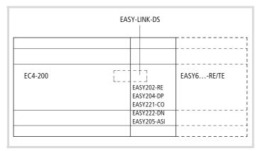
Figure 33: Connecting expansion devices with EC4-200
