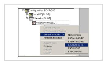
Figure 38: Selecting the expansion device
