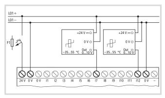
Figure 20: Temperature sensor
