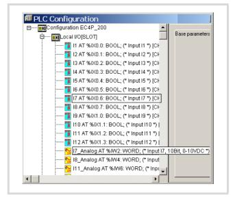
Figure 3: Selection between digital and analog input, e.g. 17
