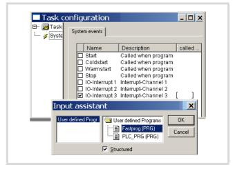
Figure 58: Allocation of Interrupt source → POU
