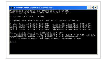
Figure 81: PING response with a correctly established Ethernet connection
