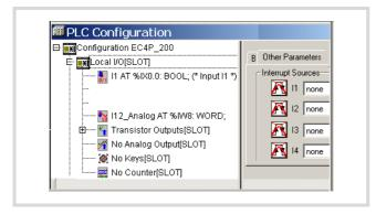
Figure 35: Selectable inputs/outputs
