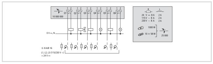
Figure 24: Relay outputs EC4P-221/222-MR...
