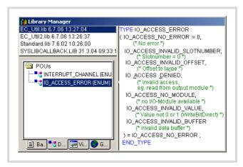
Figure 60: Return values of the EC-UTIL.Lib functions
