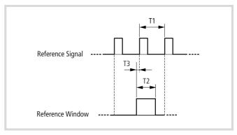
Figure 47: Relationship between reference signal and reference window
