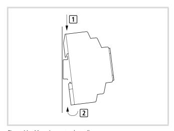
Figure 11: Mounting on top-hat rail
