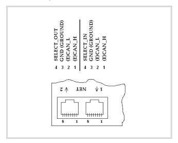
Figure 8: CAN/easyNet interfaces
