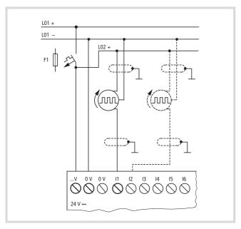
Figure 22: Connecting pulse transmitter
