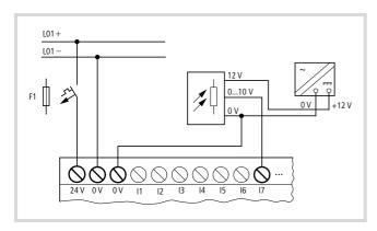
Figure 19: Brightness sensor
