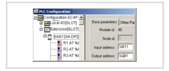
Figure 107: Setting the address ranges
